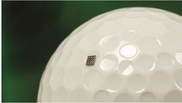
Freescale Semiconductor's Kinetis KL03 processor, shown here nestled inside a dimple of a golf ball. Freescale Semiconductor.
