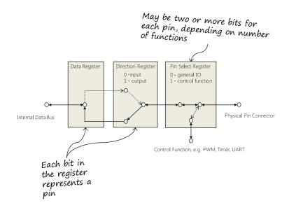
The number of, and operation of, the GPIO registers is hardware-specific and will vary from manufacturer to manufacturer; but they typically all have the same basic principles.
