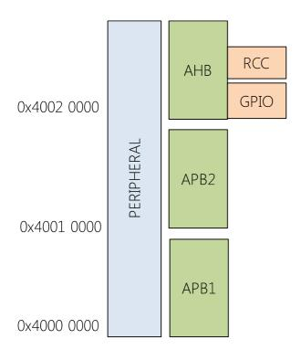
All the GPIO ports are on the Advanced High Performance bus. The addresses of the ports are shown in the table below
