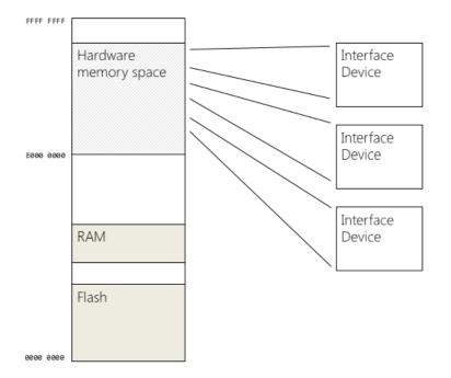
It is important to note that the two techniques are not normally found on same architecture; although for example on older PCs video ram would be memory mapped and all other I/O devices would be port I/O.
