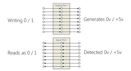
Such a mechanism would lead to a profusion of pins, and be very inflexible – there would always be a fixed number of input and output pins. In most real world microcontrollers each physical pin can be configured for a variety of uses. Usually the I/O pins are multiplexed so they can not only act as either inputs or outputs, but also perform alternative operations (e.g. transmit pin for RS232).
