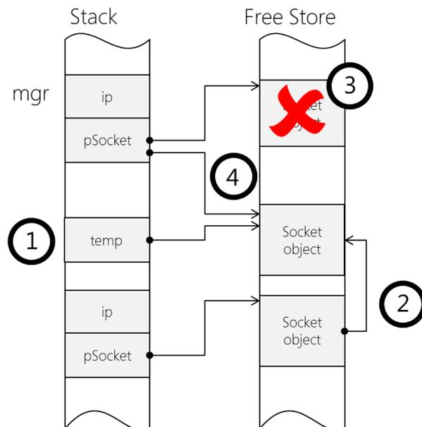
1. A new resource (a Socket in this case) is allocated. We do this before deleting our old resource just in case the allocation fails - we'd be left with a 'broken' object.
