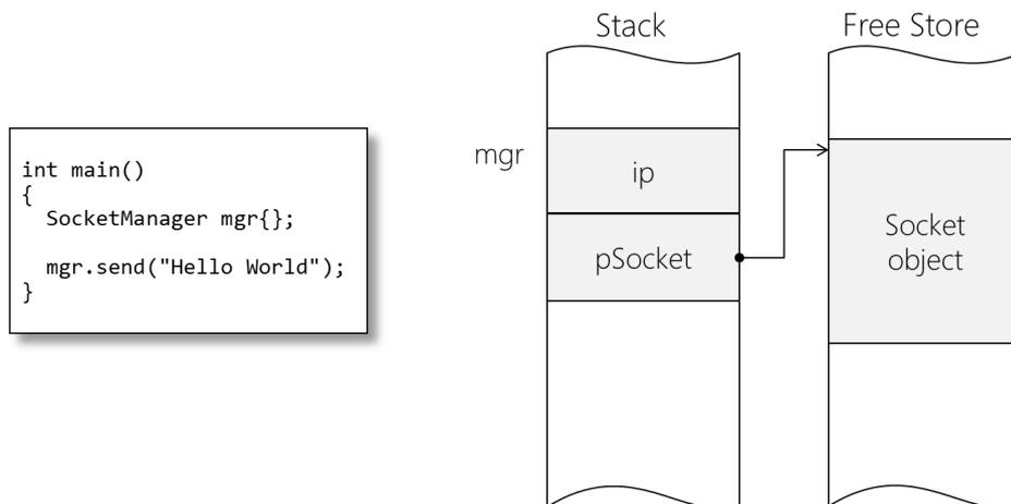
When mgr (above) goes out of scope (in this case at the end of main; but in general at the end of the enclosing block) its destructor will be automatically called. The destructor calls delete on the pSocket pointer, which automatically calls the Socket’s destructor *before* releasing the memory for the Socket.
