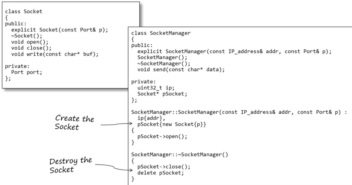
A small warning here: make sure the new and delete operators ‘match’: that is, if the resource is allocated with new, then use delete; if the resource is allocated as an array (new [ ]) make sure array delete is used (delete [ ]) Failure to do so will lead to ‘Bad Things’ happening.
