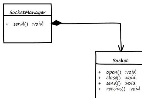
The SocketManager is responsible for the lifetime of its Socket object. The Socket is allocated in the SocketManager constructor; and de-allocated in the destructor.
