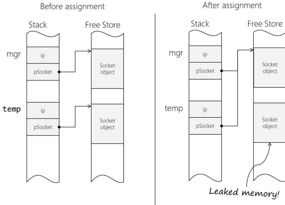
At the beginning of `func()` a temporary object is created, with its own `Socket`. `mgr` also has its own `Socket`.
